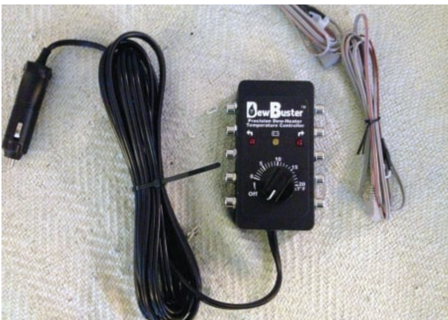
Image 4 - The new DewBuster out of the box. The kit consists of the controller, power cord and two corded temperature sensors
