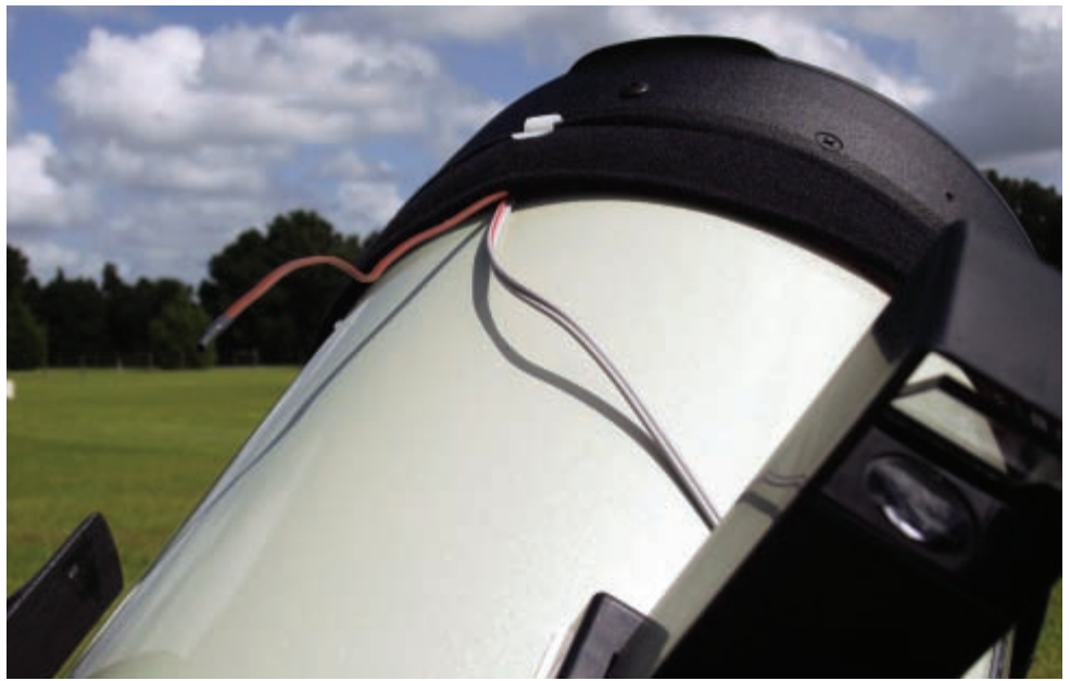
Image 6 -The DewBuster Temperature Probe Installed on Uncle Rod's C8
