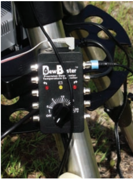
Image 5 - The DewBuster Controller Mounted on Uncle Rod's C8 Tripod
